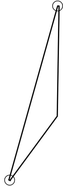
Something to remember when you are making templates; very acute angles, such as head of flying jibs and tack corners, cannot come to a point, it is physically impossible to bring cotton cloth to a sharp end as it must be turned to hide a raw edge. There should be a 'nose' of around 3/32".
